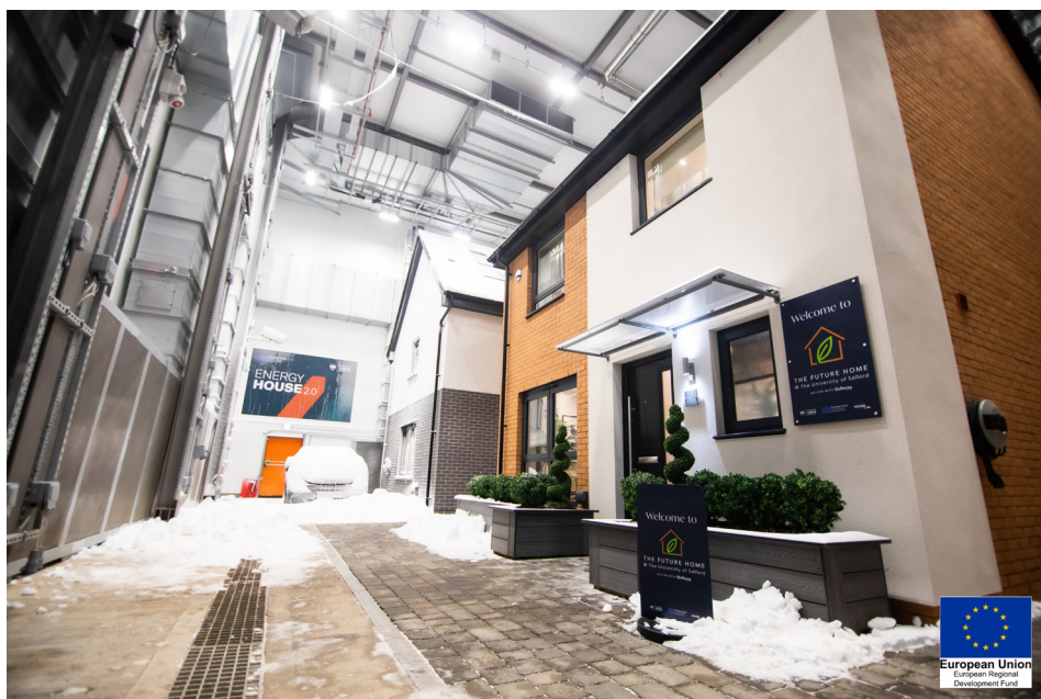
Energy House 2.0 at University of Salford. Environmental chamber for testing fully built homes for R&D purposes. (Image credit: Charles Leek)
